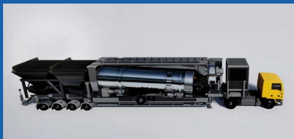
2 - Dryer, filter, cold feeders (n°4)
