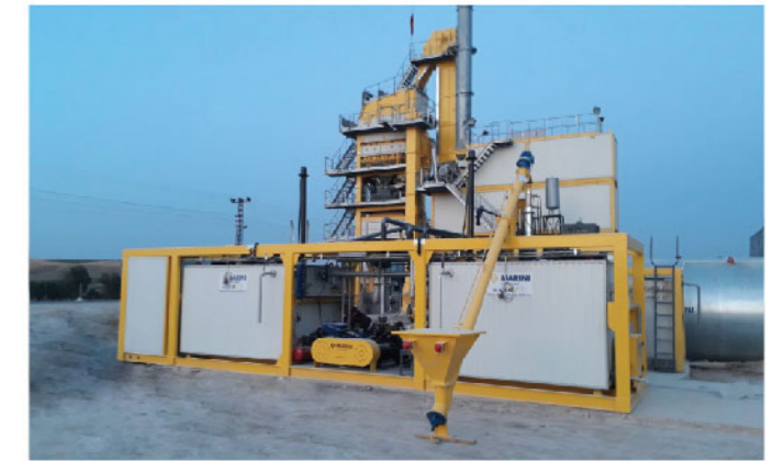
ARGENTINA - modiFALT30 PMB Plant up to 30 t/h
