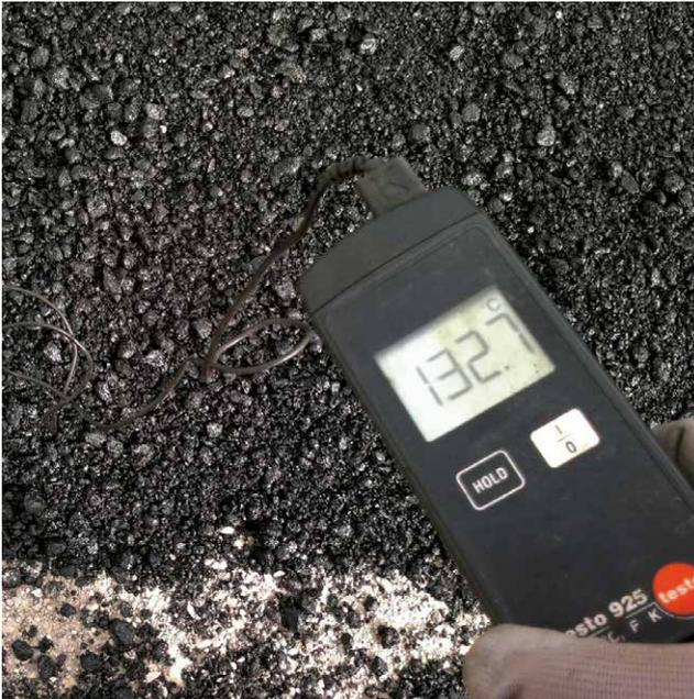
Warm Mix Asphalt (WMA) is already the asphalt mix of tomorrow. Most commonly produced at 30°C below Hot Mix Asphalt (HMA) temperatures, WMA ensures high mechanical performances similar to those of HMA, while providing a whole range of benefits:
