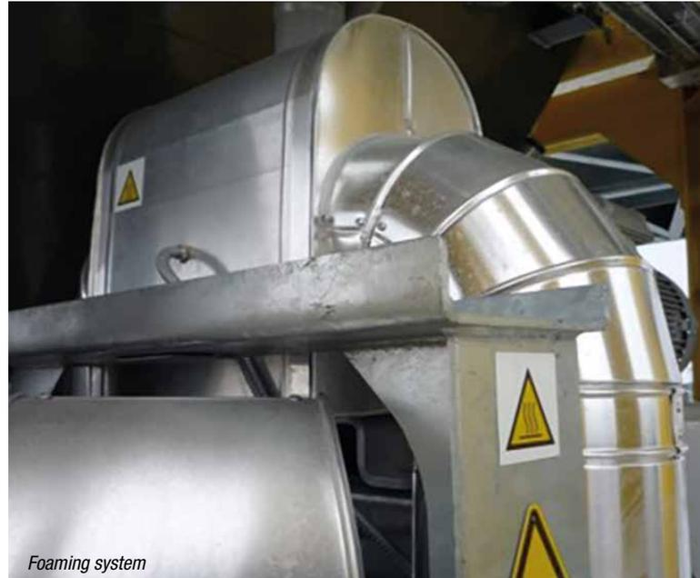
Water based WMA technology is the best performing solution, especially the micro-bubbled foam bitumen solution (with high pressure water) which offers the widest range of technical and economical advantages.
